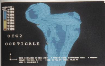
Fig. 5 and 6 - Finite element analysis picting the stress distribution of the femur cortical bone without and with a composite hip prosthesis.
