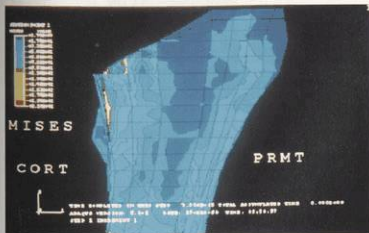
Fig. 5 and 6 - Finite element analysis picting the stress distribution of the femur cortical bone without and with a composite hip prosthesis.
