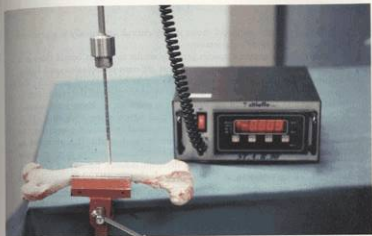
Fig. 3 - The measurement of insertion and remotion torque of coated and uncoated titanium pins.
