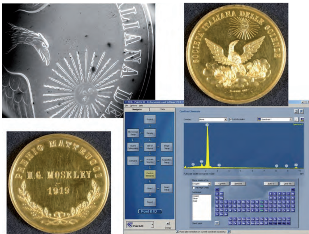
Fig. 6. Colour photographs of the front and Back of Moseley's Medaglia Matteucci along with an image of the medal taken in a scanning electron microscope and an electron beam excited X-ray spectrum, dominated by the gold M emission line (Photographs and images by courtesy of Trinity College Oxford and the Department of Materials, University of Oxford).
